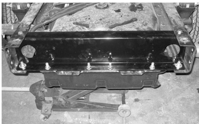
Remove support when crossmember is firmly secured.
