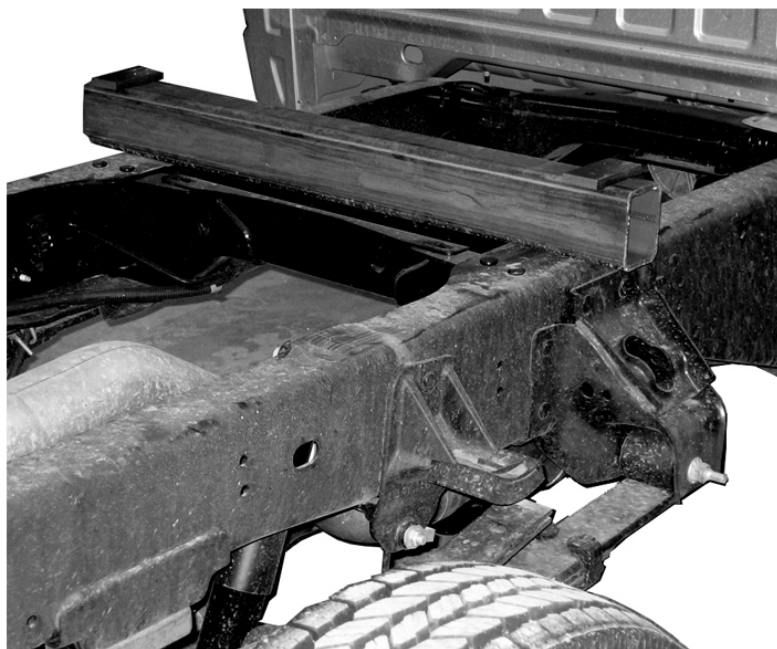
Position 3 x 4 in. beam as shown in diagram.
