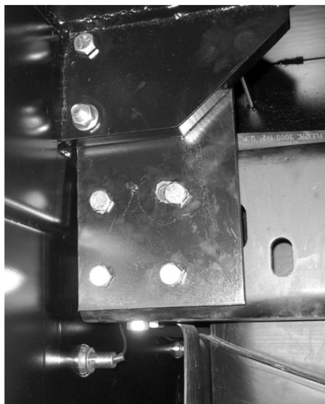
Bolt rear mounting plates to "hatchet-head" on bed and rear of truck frame.
