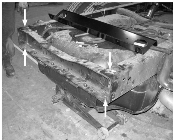
Grind off rivets and remove rear crossmember.
