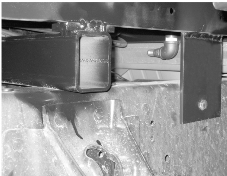
Bolt or weld mounting plates to bed and bolt to truck frame as shown in diagram. Use a minimum of six plates (three per side on front, middle and rear).
